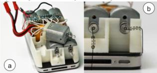
Figure 7: The *pocketOuija* mechanical design: (a) The casing contains 6 motors, 2 batteries and a *Arduino Nano*. (b) The casing implements a system of tubes that guide strings around the device.
